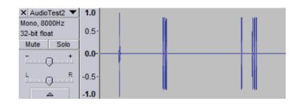
Peak level for DTMF was consistently above -2 dB on all tests
